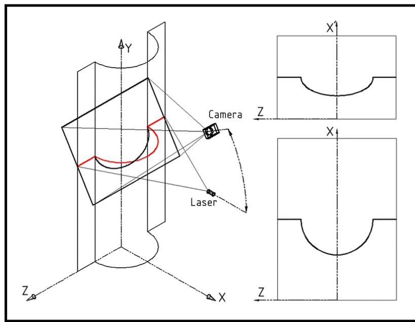
**Fig.3.** The applied method of the light cutting
