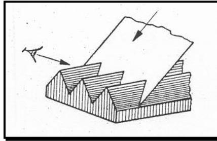
**Fig.1.** Scheme of light cutting[2]
